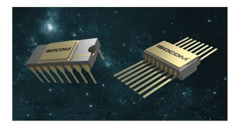
The CDL400 and CDSML400 are hermetically sealed linear optocoupler dual channel devices, consisting of an optically coupled LED with two photodiode detectors with each channel. Package styles for these devices include a 16-Pin DIP package for the CDL400 and a 16-Pin flatpack package for the CDSML400 with lead form and solder dip options available.
