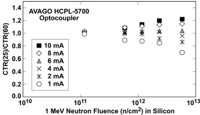
Fig. 12. Ratio of the CTR at room temperature relative to 60° C versus the radiation level for the HCPL-5700.
