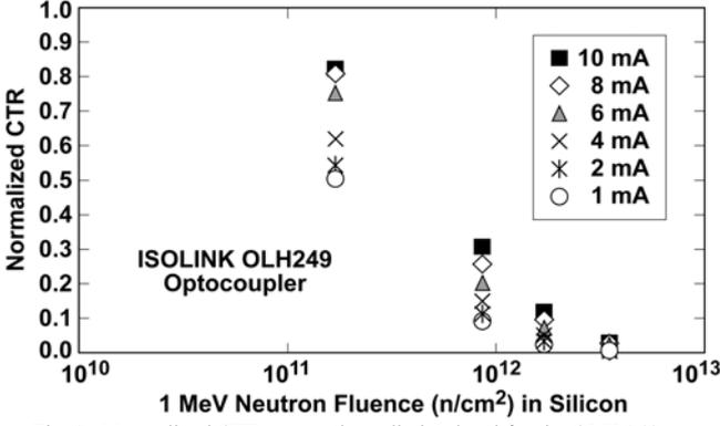
Fig. 2. Normalized CTR versus the radiation level for the OLH 249.
