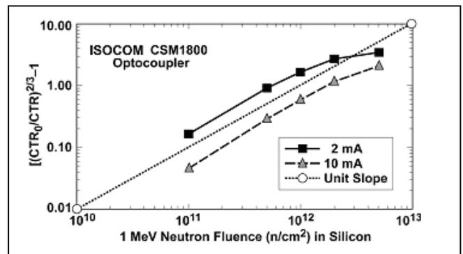
Fig. 10. Values of  $[(CTR_0/CTR)^{1/3} - 1]$  for  $I_F = 2$  and 10 mA for CSM1800.
