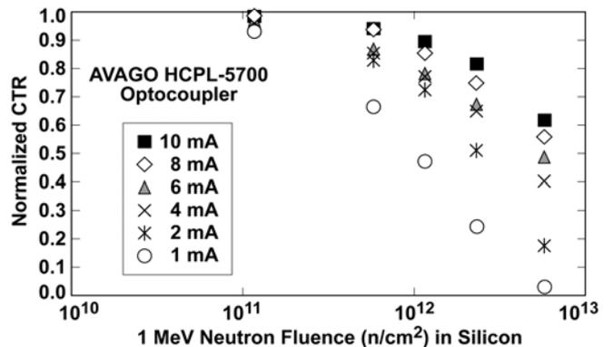
Fig. 11. Normalized CTR versus the radiation level for the HCPL-5700.
