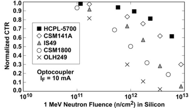
Fig14. Comparison of normalized CTR for OLH249, IS49, CSM141A, CSM1800 and HCPL-5700.
