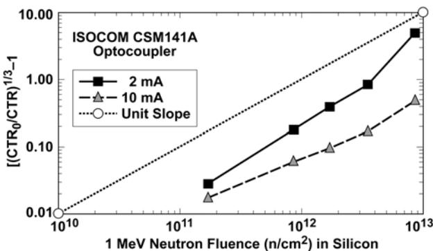
Fig. 8. Values of  $[(CTR_0/CTR)^{1/3} - 1]$  for  $I_F = 2$  and 10 mA for CSM141A.
