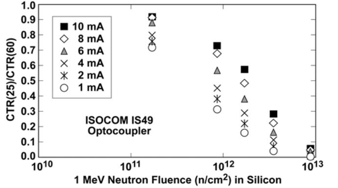
Fig. 4. Normalized CTR versus the radiation level for the IS49.
