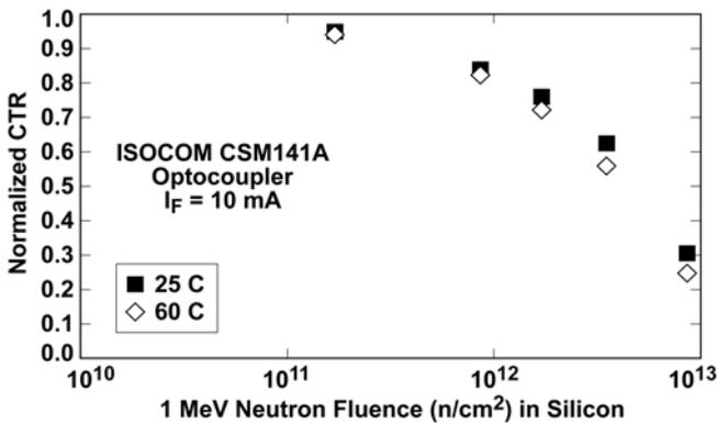
Fig. 7. Normalized CTR versus the radiation level for room temperature and 60° C for CSM141A.
