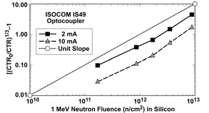
Fig. 5. Values of  $[(CTR_o/CTR)^{1/3} - 1]$  for  $I_F = 2$  and  $10$  mA for IS49.
