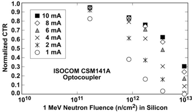
Fig. 6. Normalized CTR versus the radiation level for the CSM141A.
