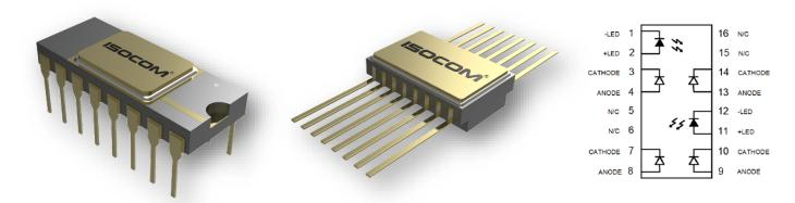
The CDL400 and the CDSML400 are hermetically sealed linear optocoupler devices, consisting of an LED optically coupled with two photodiode detectors. Package styles for these devices include a 16-Pin DIP package for the CDL400 and a 16-Pin flatpack package for the CDSML400 with lead form options and solder dip options available.
